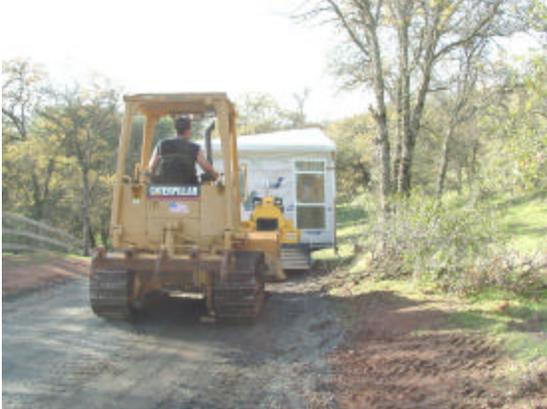
This Jade steering axle is extremely valuable for difficult deliveries. It is towed to the site, mounted under the home and provides remote control lift and steering. It even lifts differentially on side hills. Many roads that were once too difficult can now accommodate a home delivery or a larger home. This unit takes about an hour to set up or remove.
