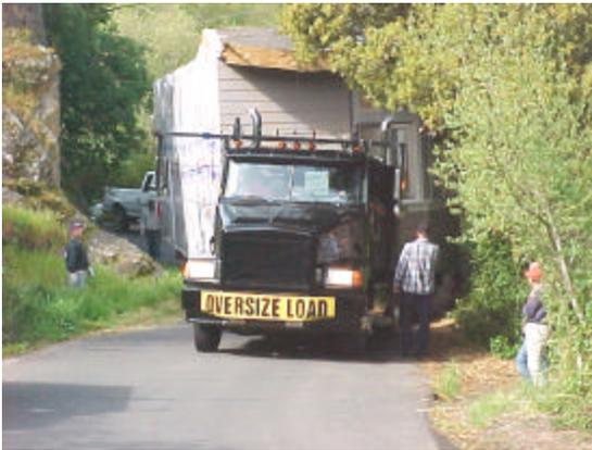
A house cat is designed especially for moving manufactured homes. It can maneuver a home down roads that are just too tight with a truck alone. Another benefit is the house cat can crawl very slowly and is smooth stopping and going. The home arrives to the building site in much less abused condition. In a tight delivery, there is no substitute for a house cat. This machine requires a competent experienced operator.
